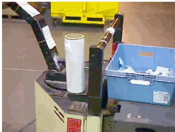
Figure 25. Example of holder on a pallet jack to secure plastic-wrap rolls.
