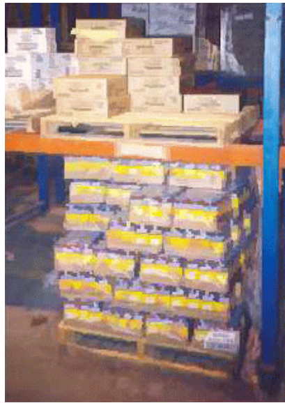
Figure 13. Tight fit of a pallet in a half-slot, making some cases difficult to retrieve and requiring selectors to bend or reach excessively.
