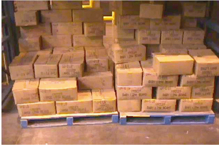
Figure 21. Pallets side-by-side in a slot, resulting in no access between pallets.
