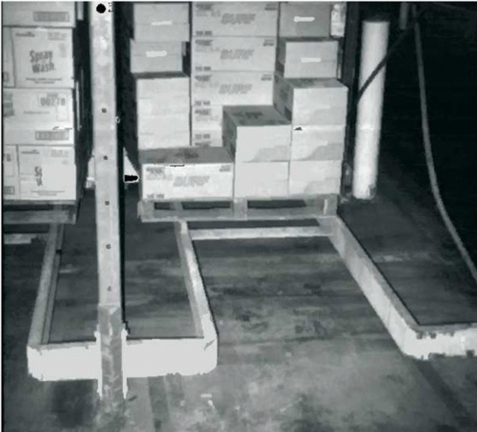
Figure 6. One method of raising pallets off of the floor, using risers in a full slot.
