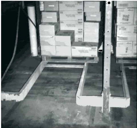
Figure 19. Risers used to elevate pallet from the floor and allow easier access to cases, but may create a tripping hazard.
