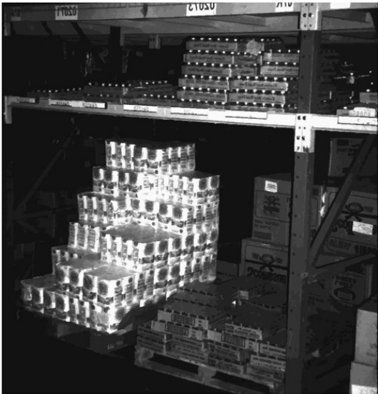
Figure 17. Gravity-fed flow racks used above a near-full slot.
