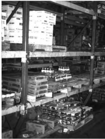
Figure 14. Example of a triple slot, which requires more extreme body positions of selectors to reach cases.
