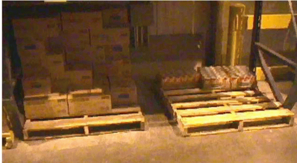
Figure 22. Pallets set apart in a slot to increase the clearance between pallets and provide easier access to selectors.
