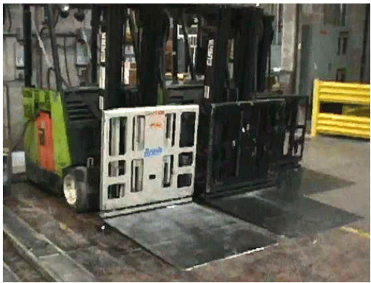
Figure 16. Load splitter with flat bed to slide under a slip sheet for moving one or more layers of cases.
