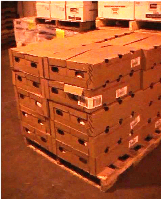
Figure 10. Handle cut-outs in cases, to ease lifting and carrying.
