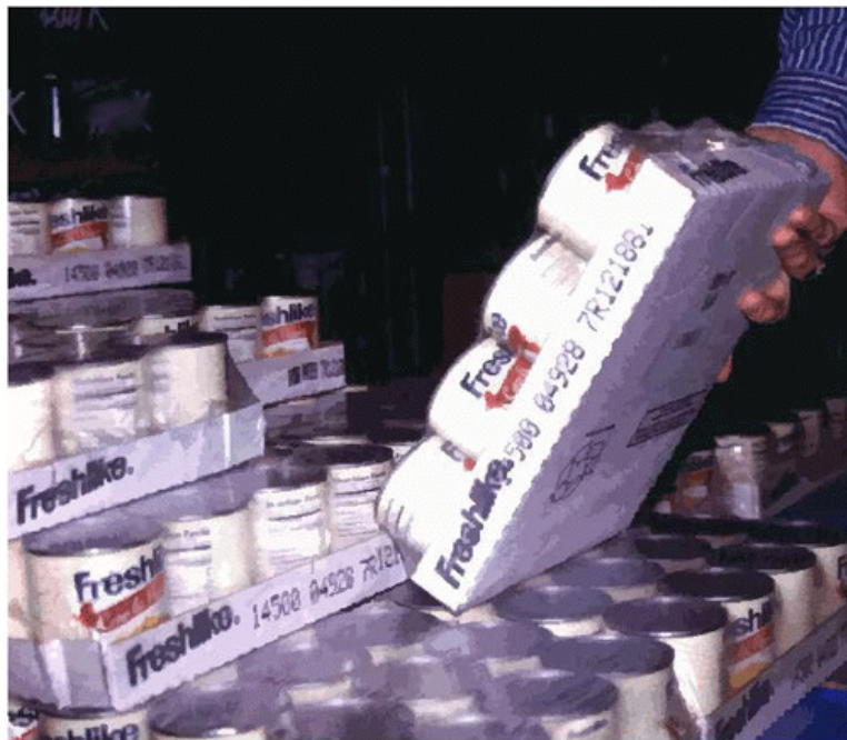
Figure 12. Tray-packs without plastic wrapped on the bottoms of the cardboard trays.
