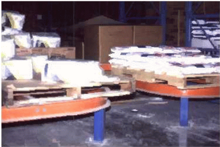
Figure 7. A second method of raising pallets off of the floor, using risers in a full slot.
