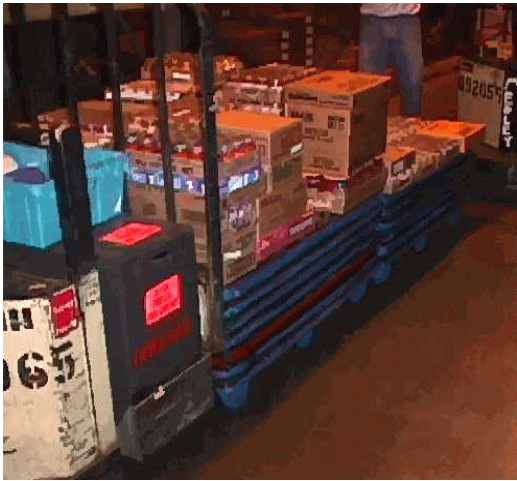
Figure 24. Stacking of empty pallets on a pallet jack, to raise the initial stacking height of cases and reduce trunk bending.
