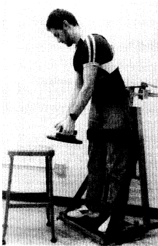
Fig. 1. A lower-body isolation structure (LBIS) was constructed to fasten the subject's legs and hips into a static position over the center of the force plate and transfer all forces and moments into the force plate. The upper-body is completely free to move. The pictured subject is also wearing a lumbar motion monitor to measure trunk motions.
