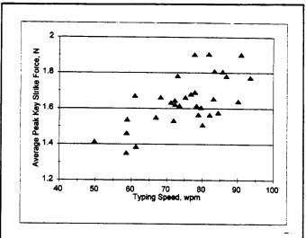
FIGURE 2. Average peak key strike force as a function of typing speed, from S5, experimental protocol
