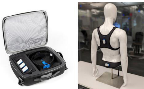
Figure 2 Motion kit, harnesses and IMU sensor configuration for low back assessment. IMU, inertial measurement unit.
